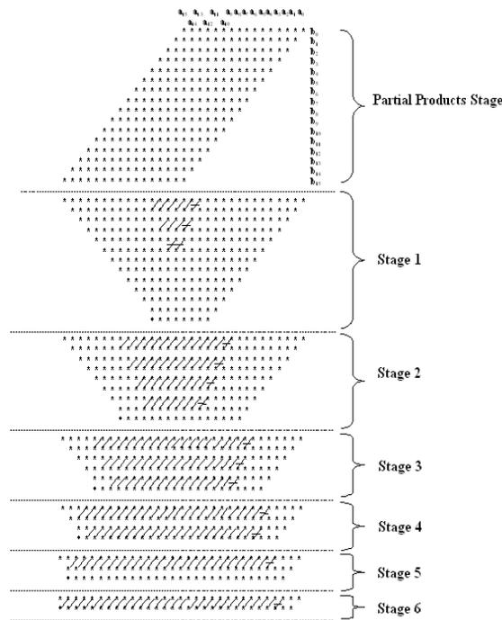
Fig 2: Dot diagram of proposed  $16 \times 16$  Dadda multiplier
