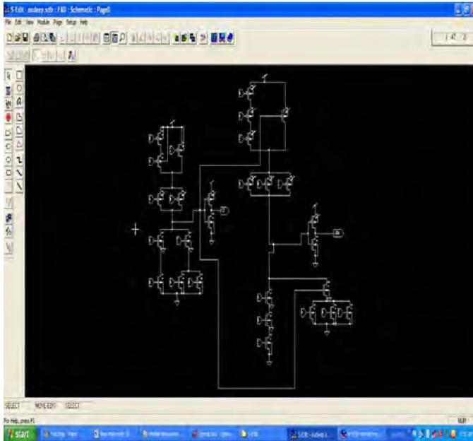
Fig 8: Schematic diagram of Full adder
