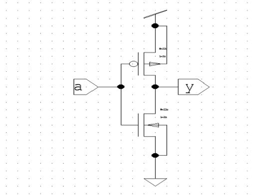
Fig 4: Schematic diagram of inverter
