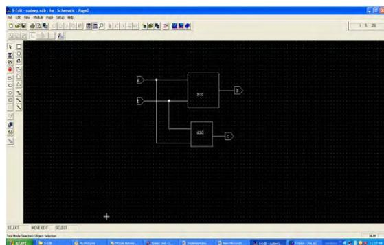
Fig 7: Schematic diagram of half adder
