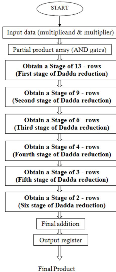
Fig 3: Flow Chart of Proposed  $16 \times 16$  Dadda multiplier
