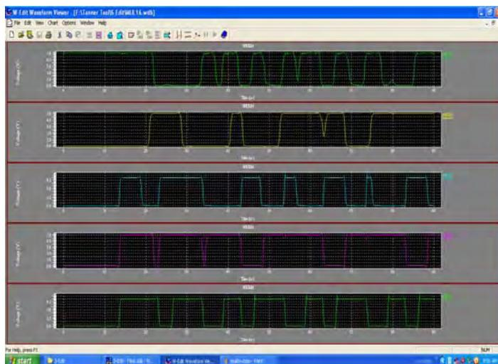
Fig 12: Output waveform of 16 × 16 array multiplier
