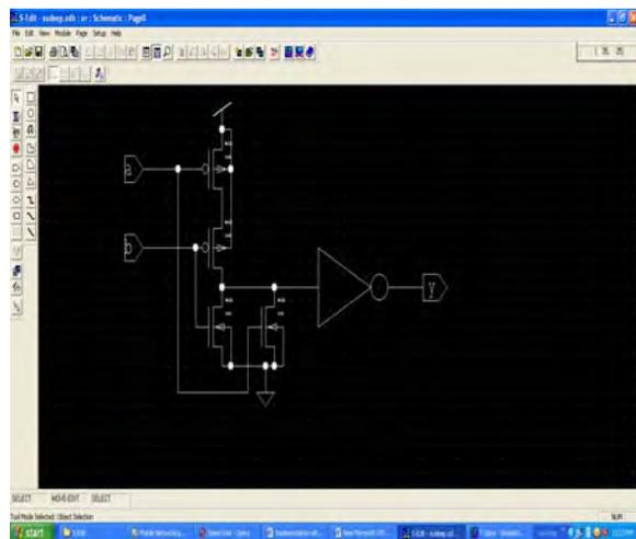
Fig 6: Schematic diagram of OR gate
