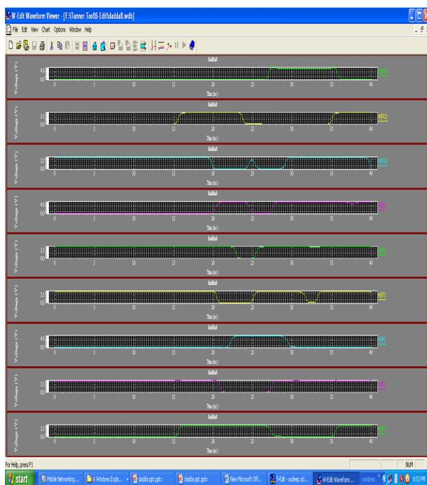
Fig13: Output waveform of 8 × 8 Dadda multiplier
