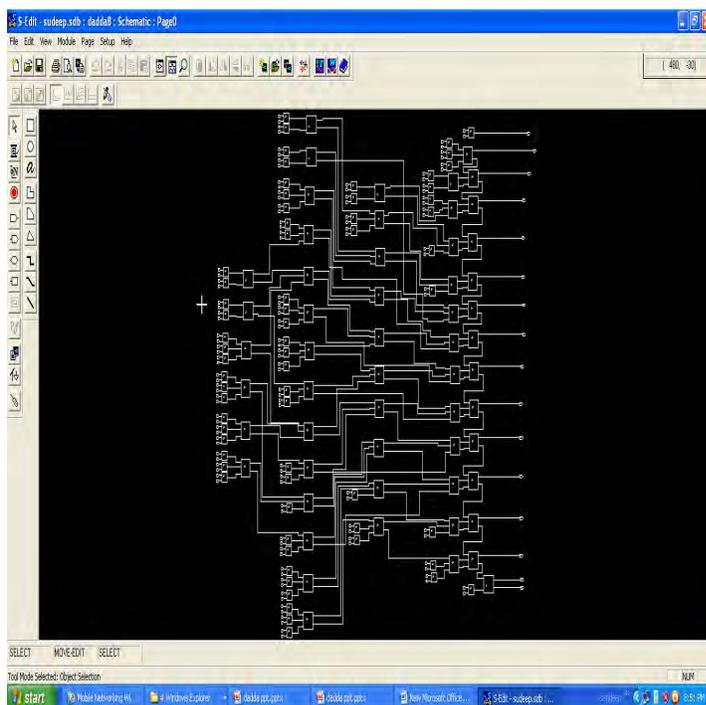
Fig 13: Schematic Diagram of 8 × 8 Dadda multiplier
