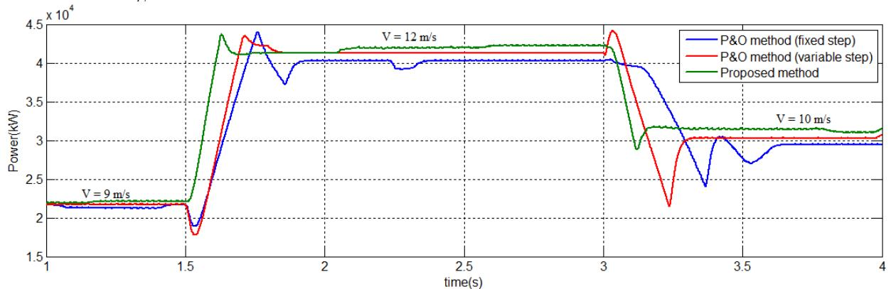
Figure 9. Simulated dynamic response of WECS output power due wind speed step change.
