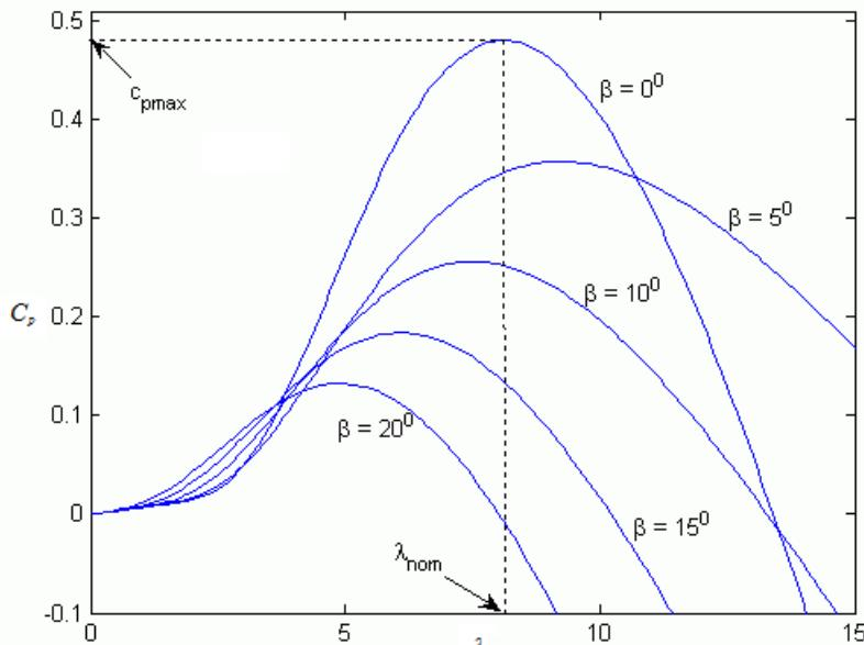
Figure 2. Typical  $C_p$  versus  $\lambda$  curve.
