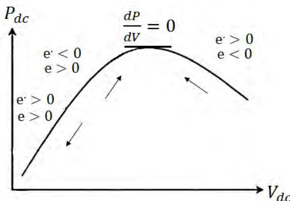
Figure 6. The P-V Curve Slope of Error and Change of Error.
