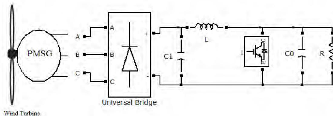
Figure 1. Wind generator system.
