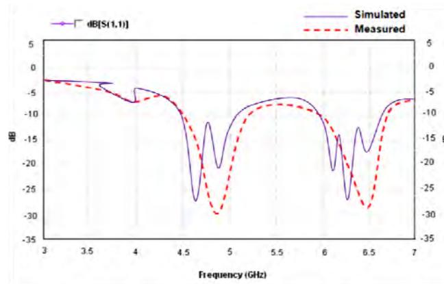
Figure 4. Return loss characteristics of a Z-U-T-S shaped antenna
