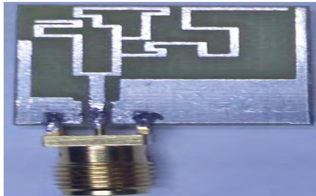
Figure 2. Fabricated Z-U-T-S shaped antenna
