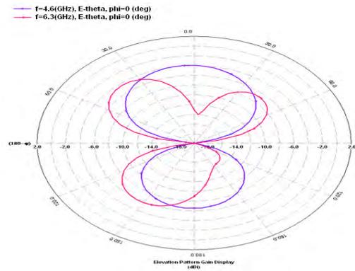
Figure 7(a). Simulated Elevation pattern (E phi at 4.6 GHz & 6.3 GHz)
