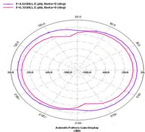
Figure 7 (b). Simulated Azimuth Pattern (E phi at 4.6 GHz & 6.3 GHz)
