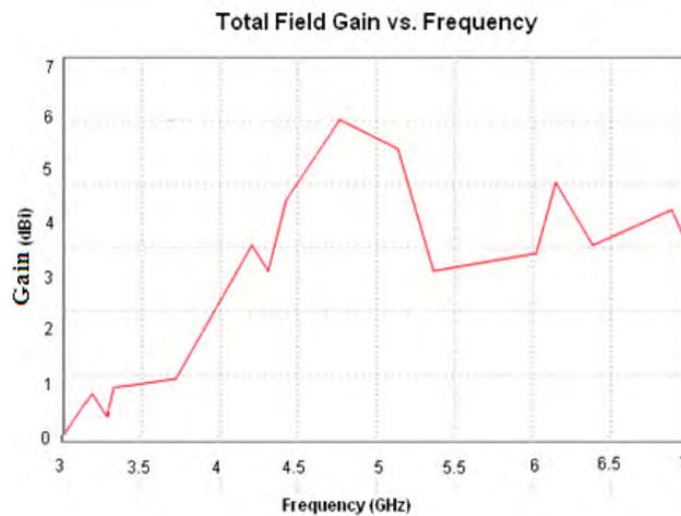
Figure 8. Gain Characteristic of a Z-U-T-S shaped antenna
