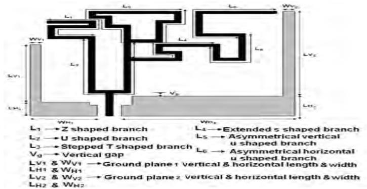
Figure 3. Parameters of Z-U-T-S shaped antenna
