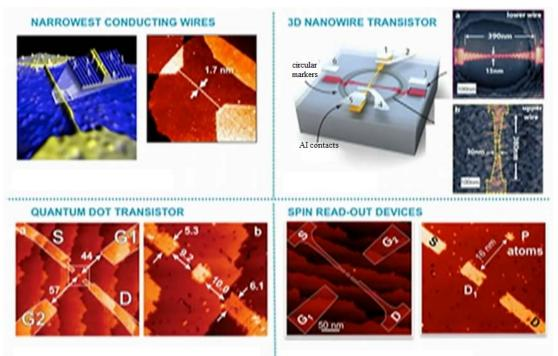
But perhaps one of the most difficult challenges for us today has been to isolate a single atom in a device. And just last year we were able to form the world's first precision single atom transistor. So that really is an individual phosphorus atom sitting in the silicon substrate, where we've aligned these electrodes to it, taken it out of the vacuum system and made contact to it. We can actually measure the electronic signature of that single atom directly.
