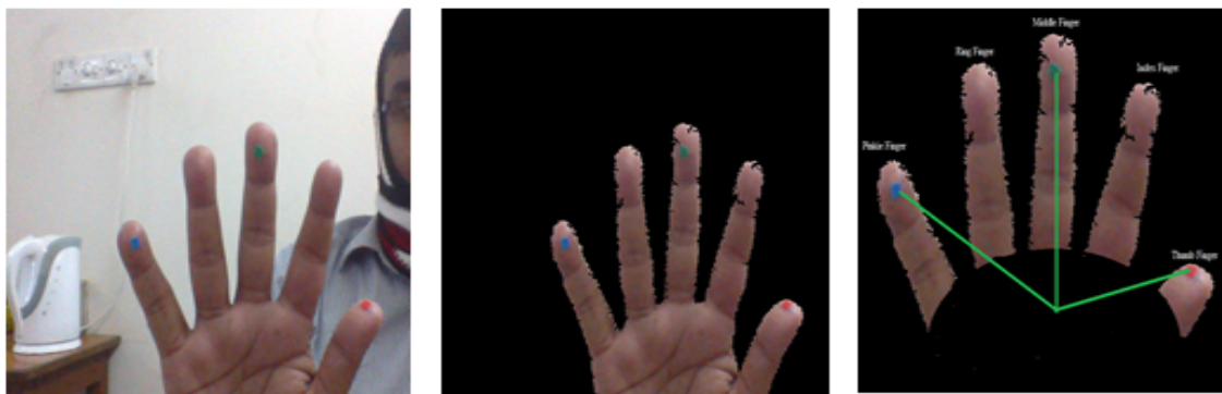
Fig-2: Webcam Image, Reconstructed Hand and Separated Fingers
