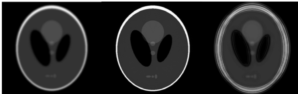
Figure 2. Deblurring on image(a) blurring with Gaussian function(PSF)(b) deblurring then super resolution (c) super resolution then deblurring (worst case)
